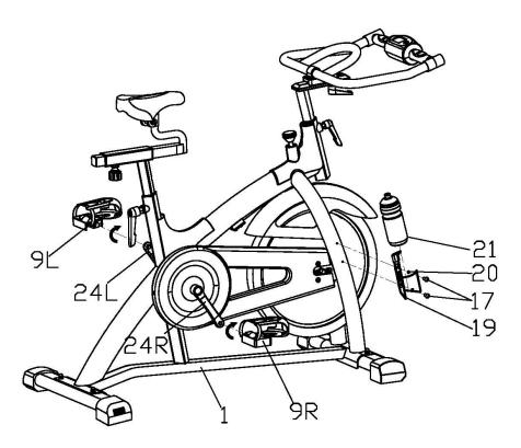
Check and tighten the screws at regular intervals, as they may loosen due to vibrations. Damage that may be caused by a lack of maintenance is not covered by the warranty.
